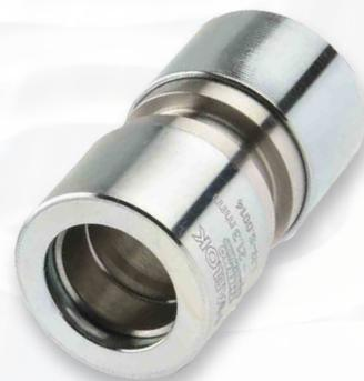
The HAELOK® THERMO fitting, type „SR“ (Straight Repair) is used for a straight connection of two district heating pipes. The fitting can be moved over the whole pipe to carry out repairs. It is especially optimized for high pull-out forces, temperature load changes and for the use according to the current specifications of AGFW FW 449. The fitting consists of three fixed mounted components; a base body and two press rings.
