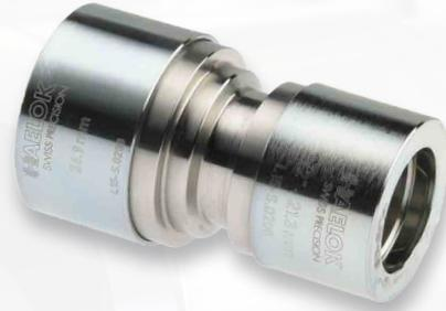
The HAELOK® fitting, type „RE“ (Reducer), is used for a straight connection of two pipes with different diameters are used. The fitting consists of a total of three permanently mounted components; a base body and two press rings of different sizes.
