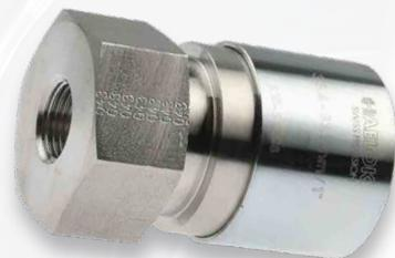
The HAELOK® fitting, type „TI“ (Thread Internal) is used to connect or extinguishing nozzles. The fitting consists of a total of two permanently mounted components; a base body and a press ring. Special designs with special threads e.g. NPT are possible.
