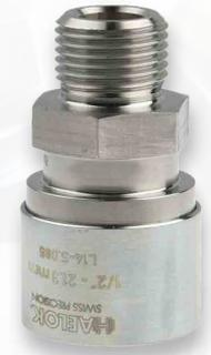
The HAELOK® fitting, type „TE“ (Thread External), is used to connect pumps or valves. In general the thread is manufactured according to type „B“ with sealing edge. The fitting consists of two permanently mounted components; a base body and a press ring. Special designs with special threads e.g. NPT are possible.
