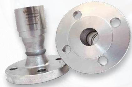
The HAELOK® fitting, type „FD“ (Flange DIN), is a detachable connection to valves, pumps and tanks. We offer from stock PN40 flange connections according to DIN 2633, standard sizes range from DN 20 to DN 50. The flanges are supplied without gaskets and fasteners. The hole pattern also fits flanges of the PN16 and PN25 series.
