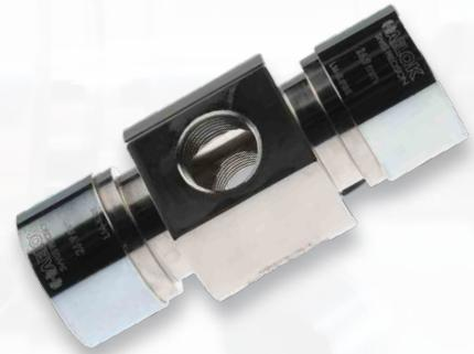
The HAELOK® fitting, type „D2“ (Distributor 2 Outlets), has two lateral outlets with G ½" thread and can be used as measuring point or for screwing in extinguishing nozzles. In connection with threaded parts TE-\_\_-G12B an outlet or crosspiece can easily be implemented. The fitting consists of a total of three fixed assembled components; a base body and two press rings.
