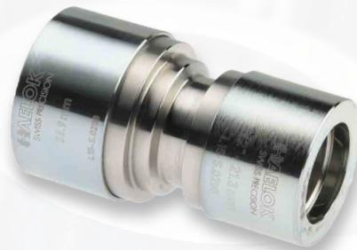
The HAELOK® THERMO fitting, type „RE“ (Reducer) is used for a straight connection of two district heating pipes with different diameters. It is specially optimized for high pull-out forces, temperature changes and for use according to the current specifications of AGFW FW 449. The fitting consists of three fixed components; a base body and two press rings of different sizes.
