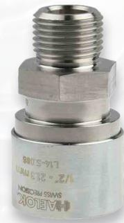
The HAELOK® fitting, type „TE“ (Thread External), is used to connect pumps or valves. In general the thread is manufactured according to type „B“ with sealing edge. For selected sizes type „E“ with Viton sealing ring is also available. The fitting consists of a total of two permanently mounted components; a base body and a press ring.
