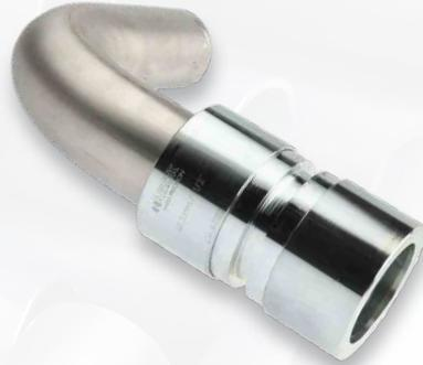
The HAELOK® fitting, type „BP90“ (Bended Pipe) is used for a connection between two pipes at an angle of 90°. The pipe is bent to guarantee a better flow and can be completed with all HAELOK® fittings. The article consists of one pipe in total.
