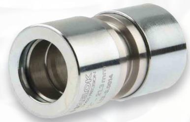
The HAELOK® fitting, type „SR“ (Straight Repair) is used for a straight connection of two pipes. Due to the missing stop, the fitting can be moved over the whole pipe for repairs. The fitting consists of a total of three permanently mounted components; a base body and two press rings.
